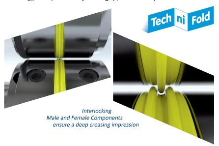
The **two-way creasing** application is performed by interlocking components. Firstly, the all-important 'U' shaped crease is formed, onto which the main fold is placed. Secondly, the **problem areas** either side of the main crease line – those prone to toner flaking after the fold is applied – are **ironed out using** a **specially profiled female receiver ring**.
