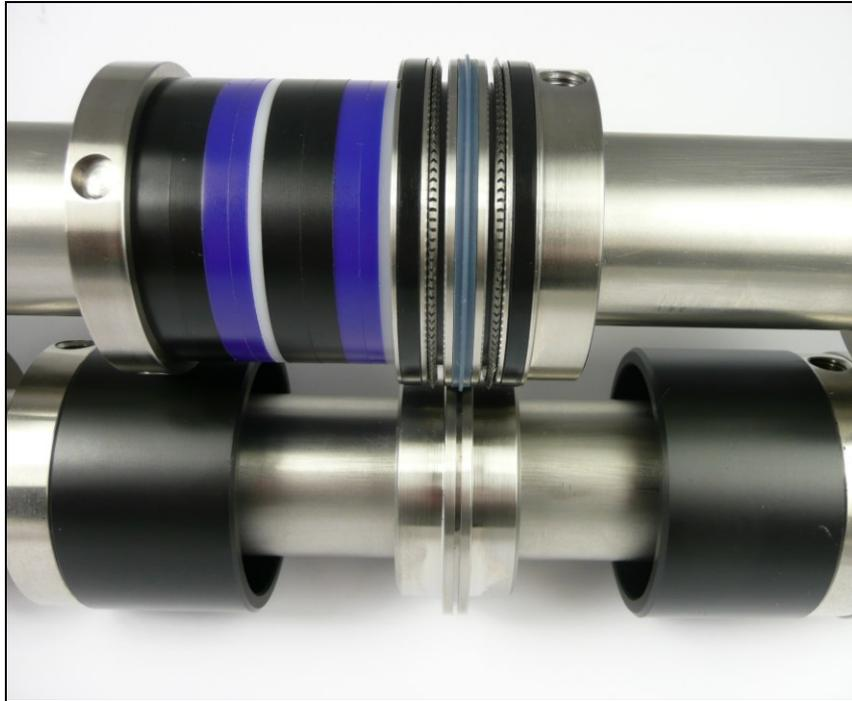
Preset the perforation blades to correct width by placing a spacer of equal width at either side of the creasing rib holder. All the exit shafts should have the fixing screws facing upwards as in the photo.
