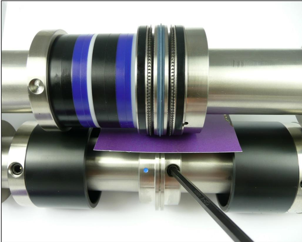
Align the female in to the centre of the gripper crease rib and insert a sheet of paper between the female and gripper crease rib. Slowly hand turn the rollers backward to enable the sheet to be fed in. This will automatically centralize the loosened female in to the optimum crease position. As the collars rotate the fixing screws will come into view, tighten the female with the paper still gripped in position.
