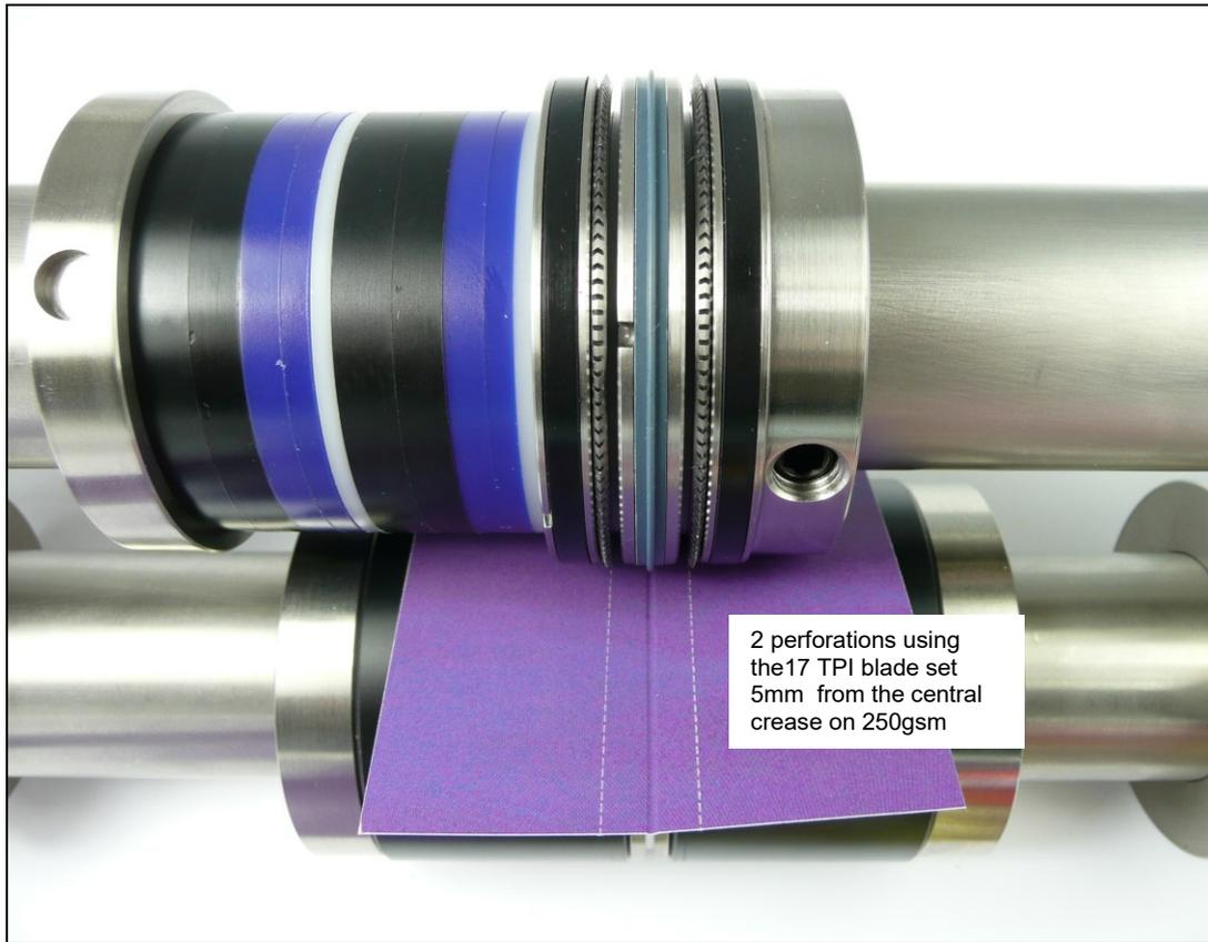
Push down the calliper pressure lever at one side of the shaft. Slide the nylon sleeves underneath the perforation blades and tighten the fixing screws.
