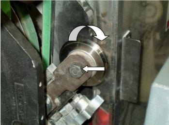
Remove the original crease unit by unscrewing the central bolt.
