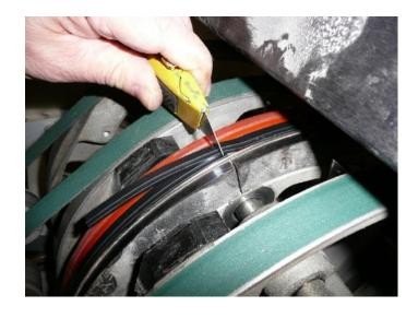
Rotate the feeder drum until the black creasing matrix over laps. Cut off the excess matrix leaving an overhang of 1mm.
