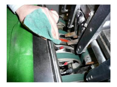
Using an abrasive cloth remove all traces of dust from the feeder drum, especially were the black rubber matrix is going to be situated.
