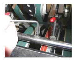
Unscrew the suction bar blanking screw (A) and the central suction arm (B) and exchange parts.
