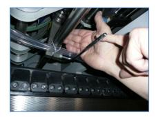
Move the creasing arm into position and tighten using a 8mm hexagon key
