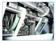
Slide on the new Technifold creasing female
