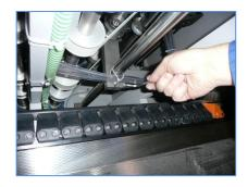
Loosen the creasing arm by using a 8mm hexagon key.
