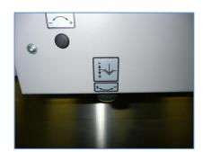
Adjust the crease depth by turning the knob
