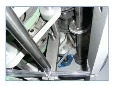
The crease unit stud with the original creasing unit removed
