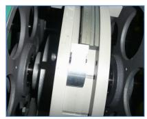
Push the 5mm black bolt through the drum and matrix holding clamp.
