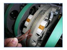
Rotate the drum and peel off the red plastic backing tape to reveal the expose adhesive
