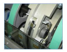
Push the crease matrix under the clamping bracket
