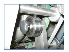
Push the female creasing arm back onto the drum
