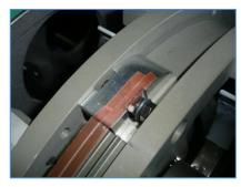
Apply 2 x strips of the red 2 x sided adhesive tape on either side of the V recess as shown
