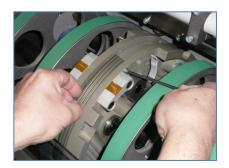
Ensure the removable creasing drum component is situated in the correct position as shown
