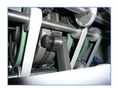
Slightly stretch the matrix as it rotates around the drum
