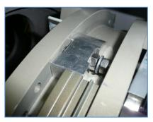
Attach the 2 x nuts and 1 x washer to the 5mm bolt at the same time
