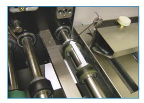
Align the new female by removing the special alignment setting tool (this is attached to the main framework situated next to the plough folding unit as shown in diagram.)
